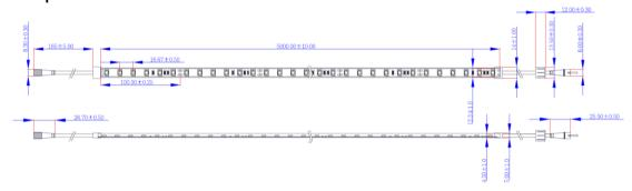
TriFlex IP65 LED Strip is supplied in 5m Reels, LED spacing 16.67 mm. Cut to length strips shorter than 5m and maintaining IP rating, are available on request.
