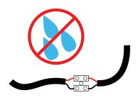
**7.** Connect fittings to drive gear. All connections should be in a dry location or made using IP67/IP68 connectors.
