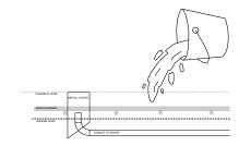
**5.** Pour concrete. Avoid filling the mounting sleeve. Clean out mounting sleeve if required.
