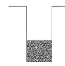
**2.** Prepare location by installing free draining material in the base of the hole to a depth of 300mm.
