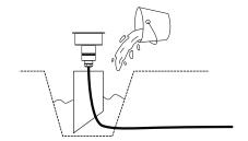
**5.** Back fill around mounting sleeve to be flush with top surface.
