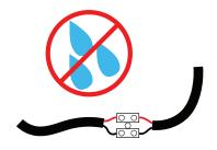
**9.** Connect fittings to drive gear. All connections should be in a dry location or made using IP67/IP68 connectors.
