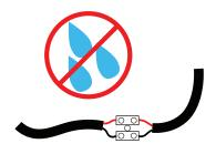
**7.** Connect fittings to drive gear. All connections should be in a dry location or made using IP67/IP68 connectors.
