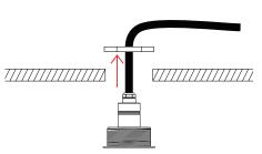
**4.** Feed the cable through the hole and locking nut and run back to a dry location for any joins. Refer Wiring Diagrams.
