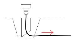
**4.** Place mounting sleeve and fitting in desired location and run cable back to dry location for any joins. Refer to Wiring Diagrams
