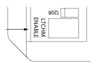
**3a.** If using a ColourTouch, turn the ColourTouch Enable switch on ONLY on the unit directly connected to the Colour Theme.
