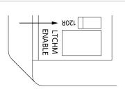
**4a.** If at the end of the DMX network, enable the 120R Termination resistor.
