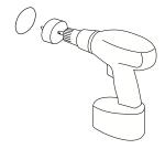
**2.** Cut a hole in the panel 15.5mm to 18mm. 15.5mm will create a friction fit.
